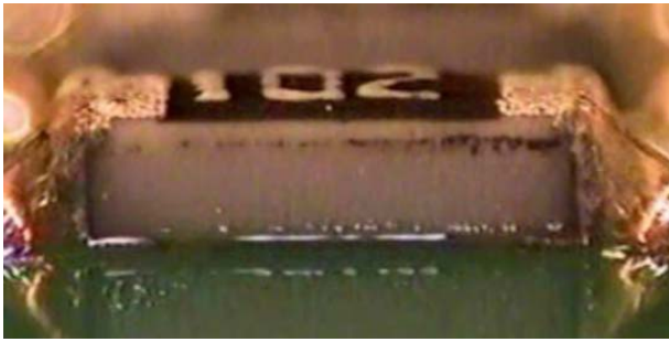
Figure 1: Flux residue trapped under component
